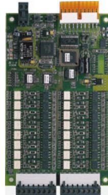
EC-Light-Input is a LONWORKS lighting controller designed to meet the requirements of any commercial or industrial application. EC-Light-Input is a networked lighting controller which interfaces with the LONWORKS network and its HVAC subsystem, providing an integrated energy management system.
